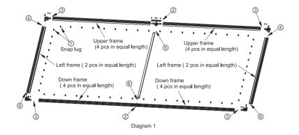
1. Please put the snap lugs into lug's slot of frame (see diagram 2) according to the Nos. of holes in the screen fabric.
